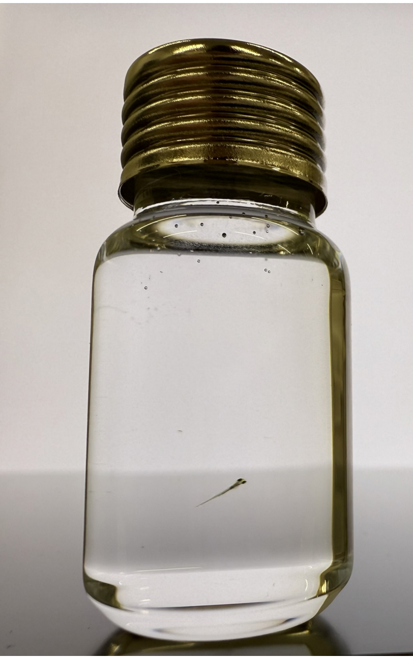
Picture 3: Glass vial design with test solution and embryo
