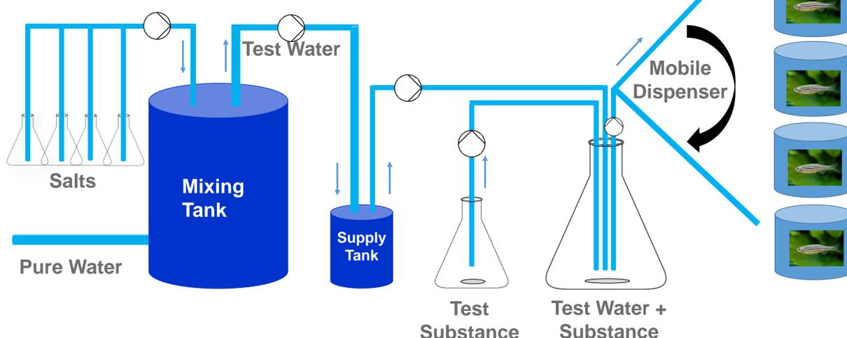
**Picture 1:** One of the flow-through systems. Control and five treatments
