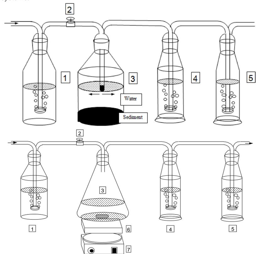
(1) Water to moisten incoming air. (2) Valve to adjust the air flow. (3) Metabolism flask containing sediment and overlaying water (OECD 308) or Erlenmeyer flask containing natural water and eventually suspended sediment (gently stirred, OECD 309). (4) Ethylene glycol trap for org. volatiles. (5) 2N NaOH trap for <sup>14</sup>CO<sub>2</sub>. (6) Insulating foam. (7) Magnetic stirrer
